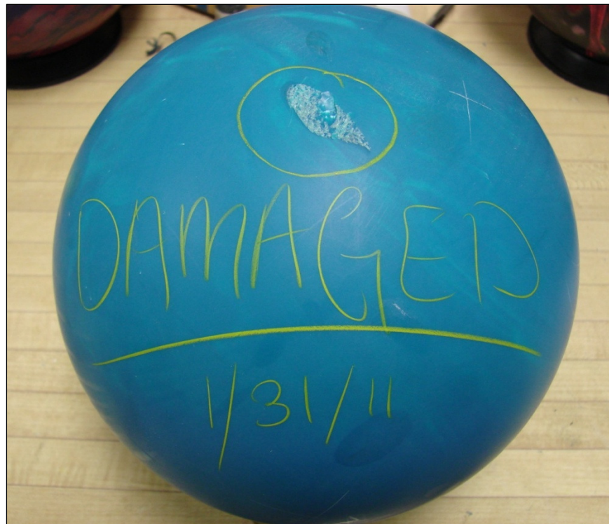
Figure 5 - USBC Static Weight Study test ball that was damaged after jumping the ball track for the ball return and colliding with the support structure under the lanes.
