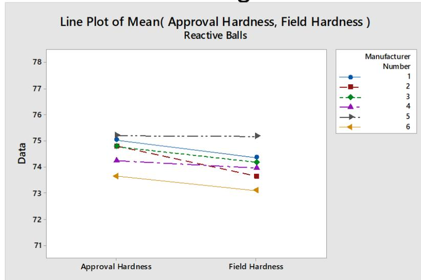
USBC monitors the hardness of approval samples and, while the data shows reactive balls have been approved at a stable level of hardness, the manufacturing target for urethane has been on a downward trajectory over the past couple of years.
