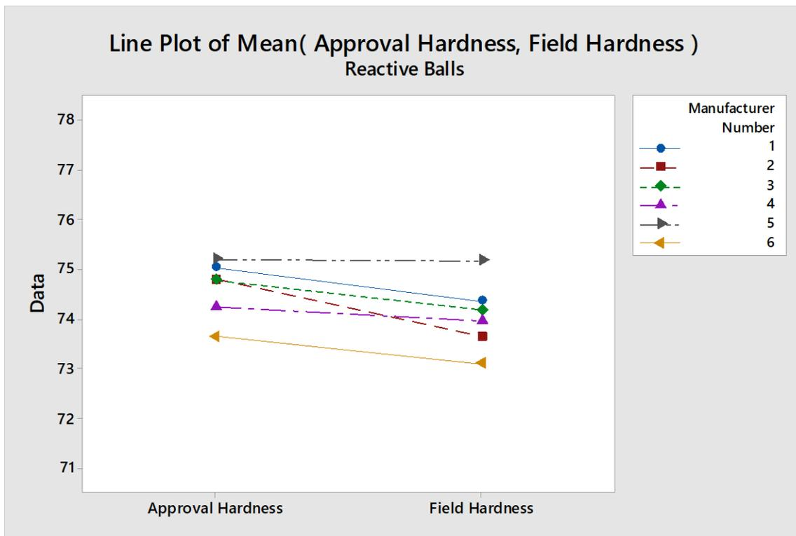
The largest difference was 1.2 points softer for manufacturer No. 2, and the smallest difference was 0.0 points different for manufacturer No. 5.
