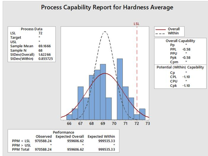
The other 85 urethane balls tested were considered “hard” urethane balls and just over one percent of these balls tested less than 72D.
