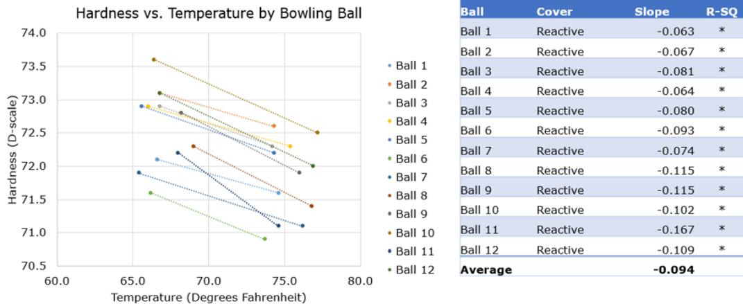
Temperature and humidity are two factors that can impact a bowling ball's coverstock. For the field tests conducted at the U.S. Open in Lincoln, Nebraska, and World Series of Bowling in Las Vegas, bowling balls were subject to different temperatures and humidity before they were submitted for testing.
