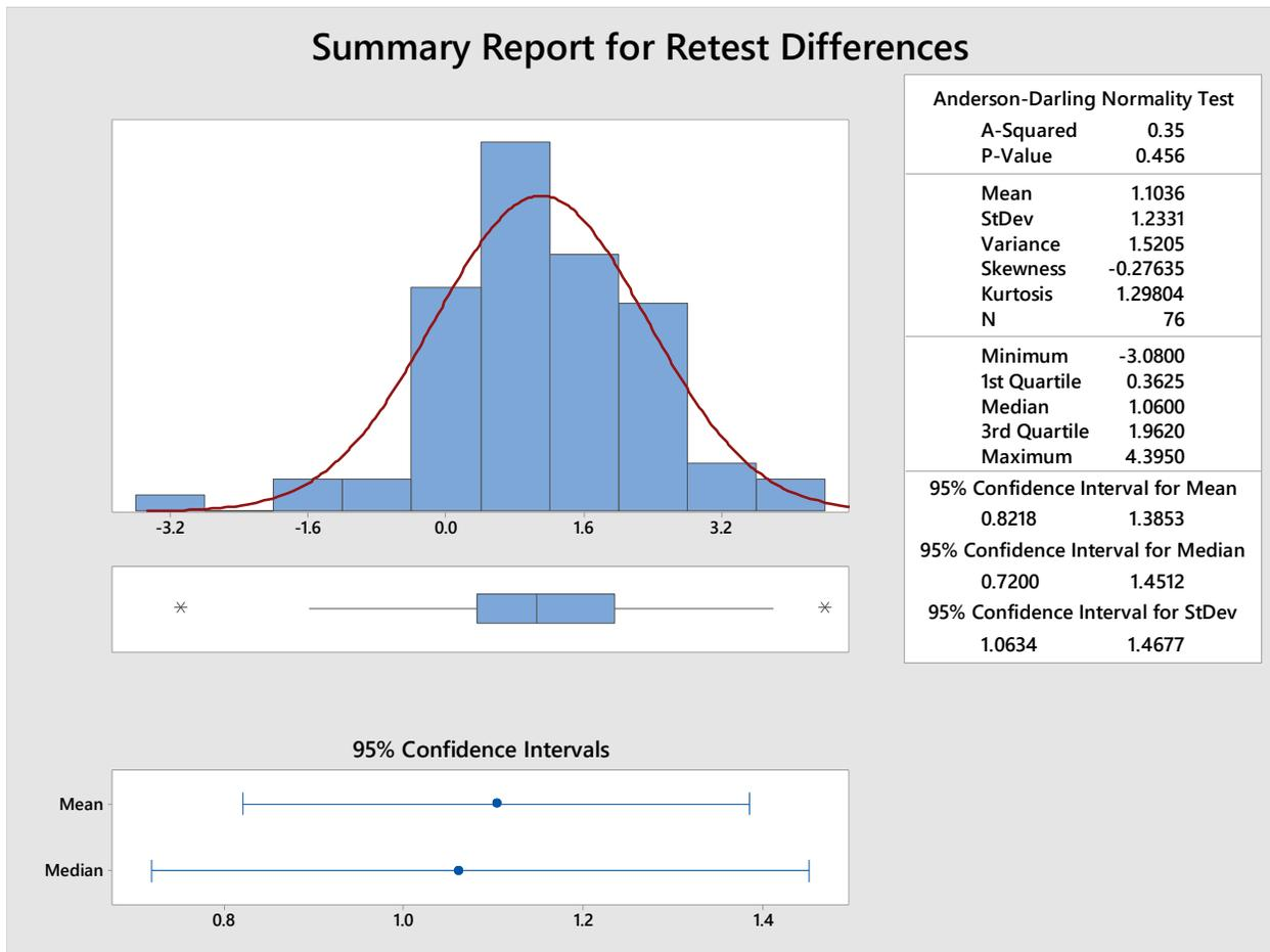
Note: Negative differences mean the ball measured harder on the second test, and positive differences mean the ball measured softer on the second test.
