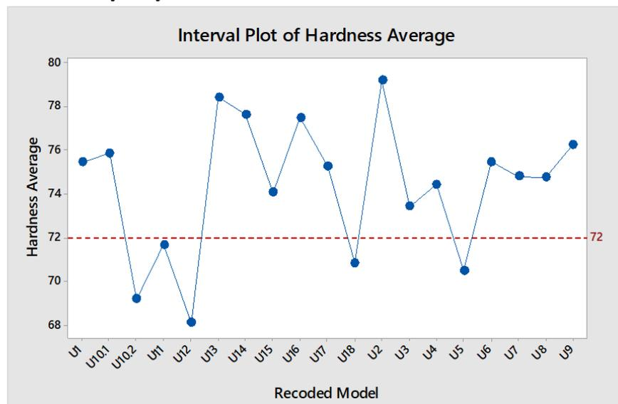
The five models comprised 68 of the 153 urethane balls tested. The field test showed 96 percent of these “soft” urethane balls tested less than 72D.
