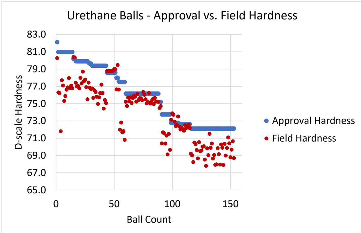
Most urethane balls drop significantly from their approval hardness, but two or three models seem to stay relatively close. Reviewing the approval data shows the models that matched closer to their approval numbers had oil absorption times of less than one hour. The fact the balls absorb oil is an indicator these balls are more of a weak reactive design, rather than a pure urethane.
