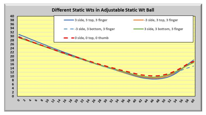
One finger weight ball hooked more than the 0-static weight ball and 3 hooked less. Some had more entry angle than the 0-static weight ball and some had less. Finger weight does not have any consistent trend.
