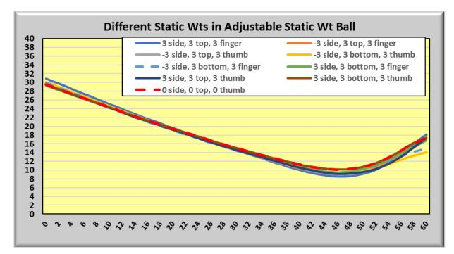
The red dotted line is the 0, 0, 0 oz. static weight ball (base line drilling). This will be used as a reference line in all attached charts to follow in this report.
