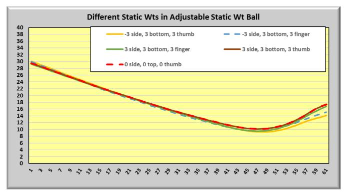
All combinations with 3 oz. of bottom weight hook the same or less than the 0-static weight and had the same or less entry angle.
