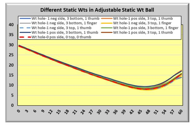
The red dotted line is the 0-static weight ball. Below is the summary data for all balls. A quick look at the ball paths (chart above) and they appear similar except for the ball with a weight hole and -1 oz. side weight, 3 bottom and 1 thumb which hooked the least. Below we isolate this ball vs the 0-static weight ball and this ball just stops hooking on the backend.
