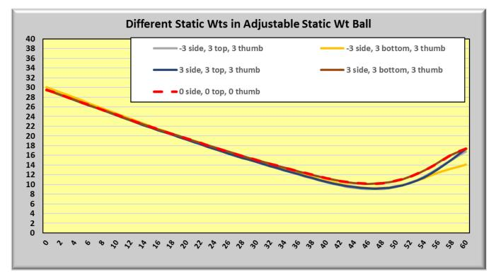
All the thumb weight balls hooked the same or less than the 0-static weight ball. Some had more entry angle, and some had less.
