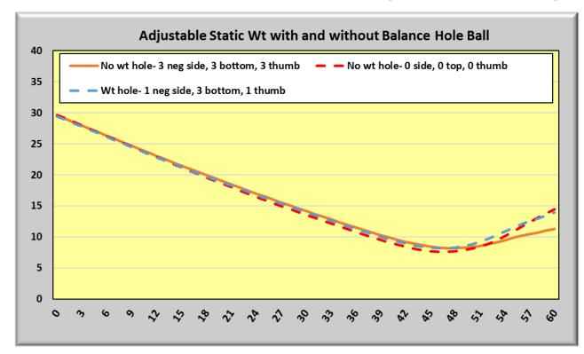
The two balls that hooked less than the 0-static weight ball, both had negative, bottom, and thumb with one having a weight hole with legal static weight and one having no weight hole with 3 oz. of imbalance in all directions.
