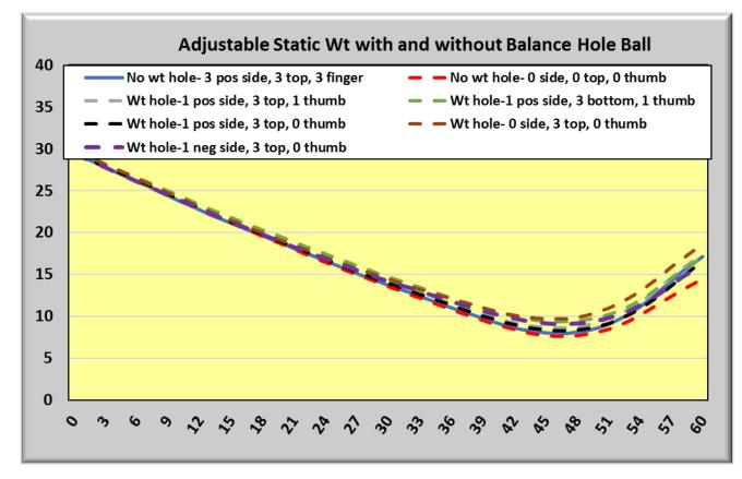
Most hooking balls were a combination of two balls with balance holes and legal static weights along with a ball without balance hole and 3 oz. static weights in the positive/ top/ finger static weight combination.
