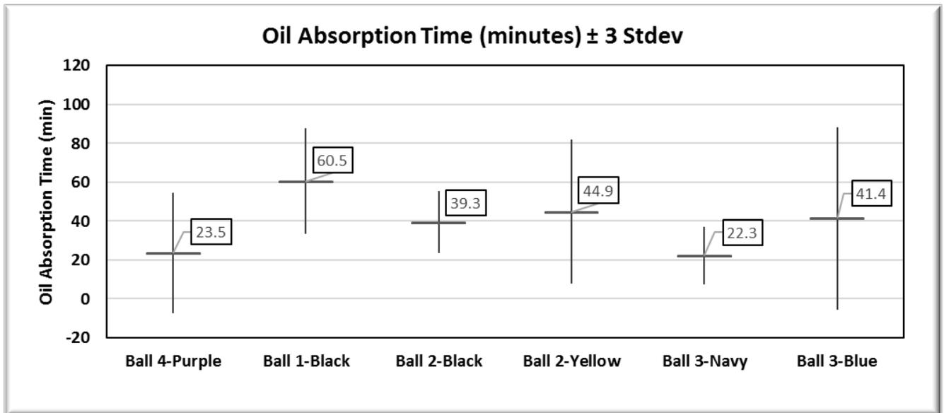
Ball #3 coverstock had a small range in the weight gain test (see chart below), but it has a consistent oil absorption time for the navy color and a wide range for the blue color (chart above).
