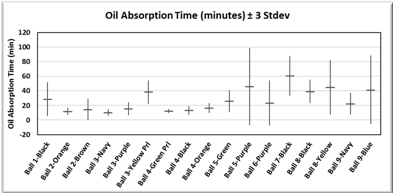
This chart (above) shows the average oil absorption time for the 10 separate tests on each color along with the range for  $\pm 3$  standard deviations. Some ranges are very small (the overall height of the data point) and others are very wide (tall heights).
