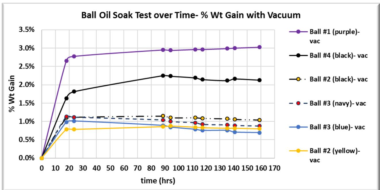
Four coverstocks increased their weight by approximately .75-1.0%. One coverstock gained about 3% in weight. Ball #4 coverstock increased its weight over a 90-hour time frame, where most other coverstocks had little, if any, weight gain after the initial 20-22 hours.
