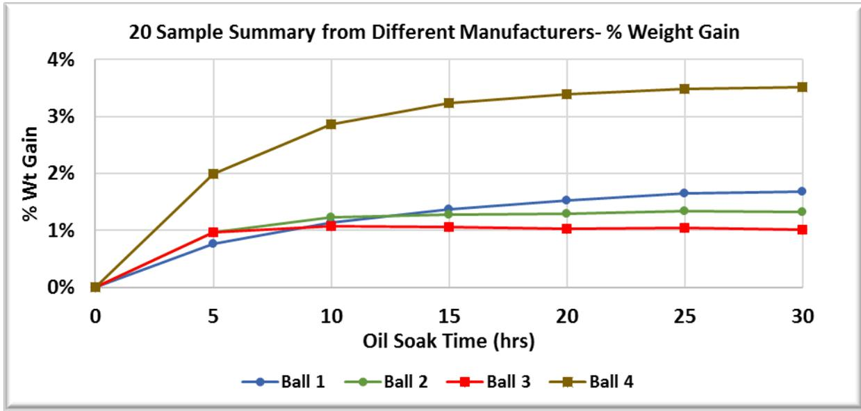
All the charts below show the repeatability between the “oil soak/weight gain” test and the “oil drop soak in time” test.
