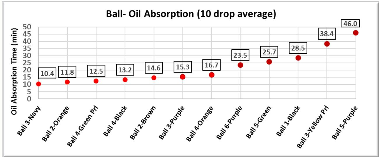
There were some large variations in oil absorption times in different colors of the same ball. This might have to do with adjustments made during production to create the color pattern in a ball with multicolor coverstocks.
