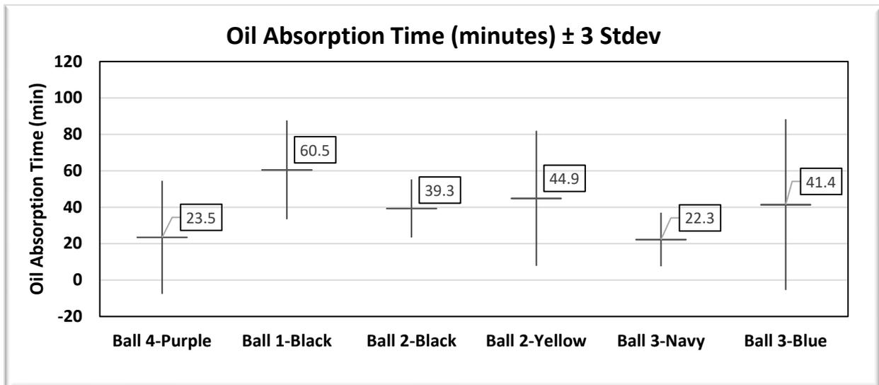
Ball #3 coverstock had a fast oil absorption time for the navy color (22.3 min) and a medium slow time for the blue color (41.4 min). In the oil soak test, this ball had the least weight gain (1.0%).
