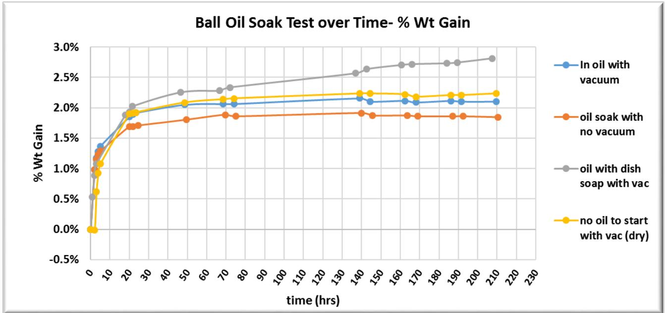
These initial tests used pieces of a production ball coverstock, the weight gain was about 1.7-2.0% after the first 20 hours in the mineral oil. After the initial 20 hours, there was little change in the weight, except for the one in the mineral oil with a few drops of dish detergent. Surfactants (dish detergent) might reduce the surface tension which makes it easier for the oil to seep into the pores in the coverstock.
