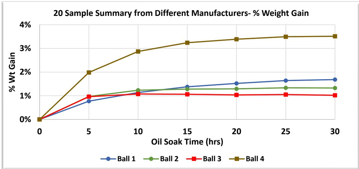
This chart is taking the total weight from all 20 samples before the test and determining the % weight gain for all 20 samples over time.
