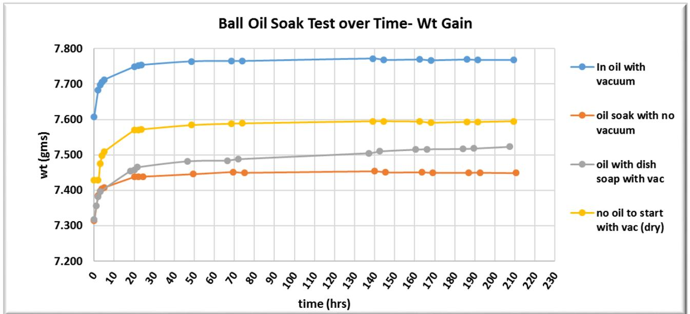
There is a rapid increase in the weight for the first 20 hours, and then the weight gain levels off. The one test with oil and dish soap (grey line in chart) did continue to increase in weight throughout the test period (210 hours).
