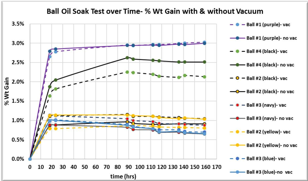
We can physically observe the vacuum draw air out of the coverstock sample by seeing air bubbles rising from the sample and floating to the top of the oil; but, in many cases, the oil absorption rate is the same with and without the vacuum assist. Therefore, we do not need the vacuum to conduct the oil absorption test.
