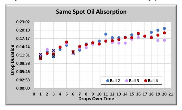
Again, the marked "X" points represent the first drop of a new day meaning two drops were taken the first day, three the next, and the remaining 15 drops taken the last day. The three first drops of the day are the shortest drop durations for the day as duration times only increase from there. All three balls also seem to follow the same trend throughout the 20-drop test.
