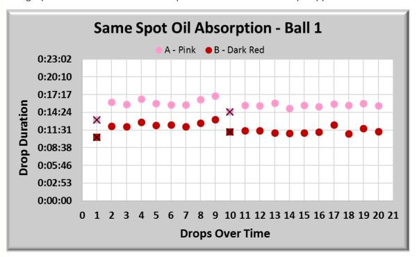
All data points represented by a box with and "X" through it indicate the first drop taken on that day. This means drops 1-9 were recorded on one day and drops 10- 20 were taken on a second day. It is important to notice that both balls, although they are two separate balls and colors, show the same relative patterns throughout each day. In all cases shown here, the first drop is a shorter duration
