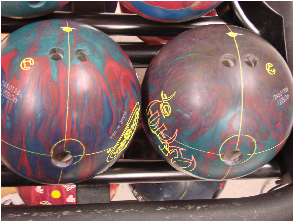
Figure 1: Photos of the positive CG ball and negative CG balls used in the test.
